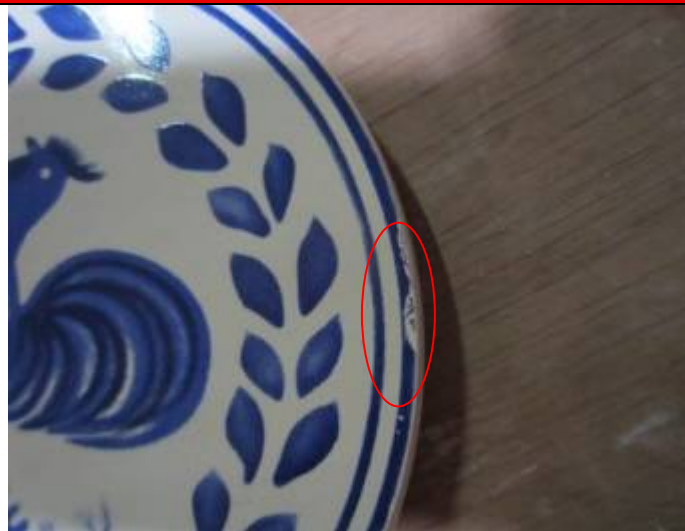
Decoration was not fully and poor painted
