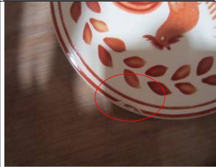
Decoration was not fully and poor painted
