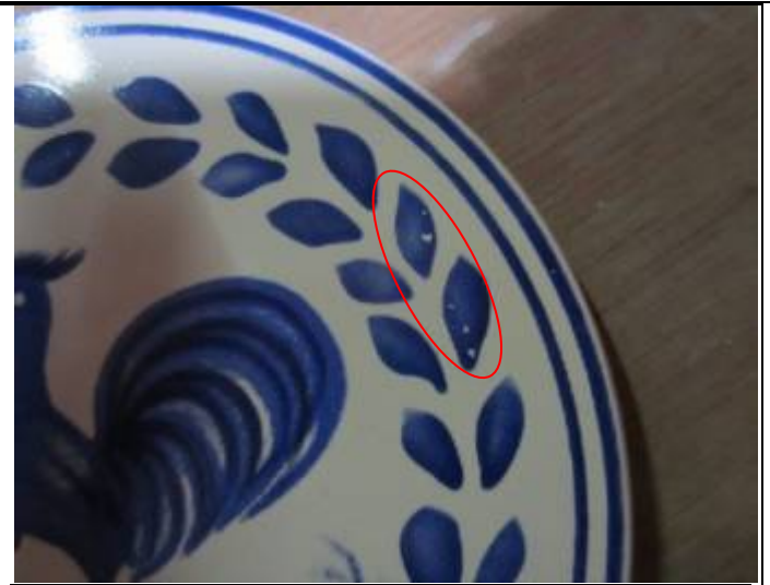
Decoration was not fully and poor painted
