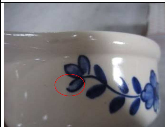
Decoration was not fully and poor painted
