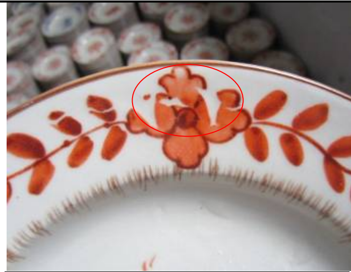
Decoration is not fully painted
