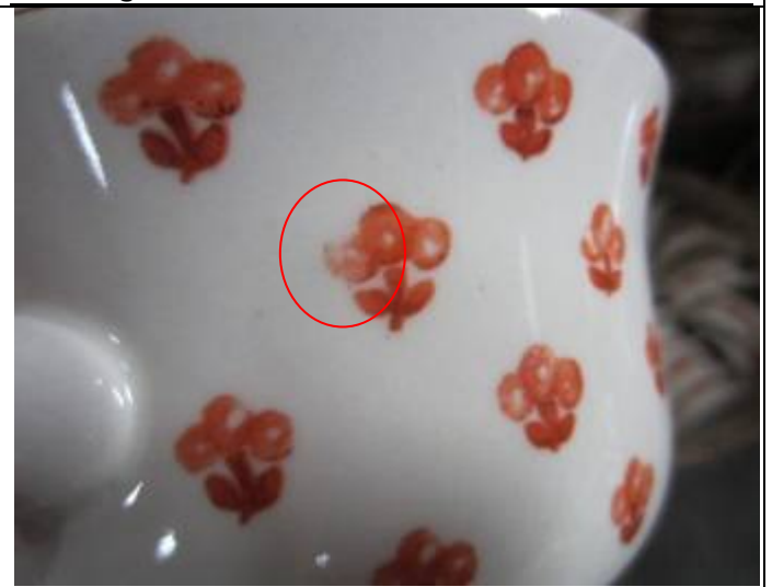
Decoration was not fully and poor painted
