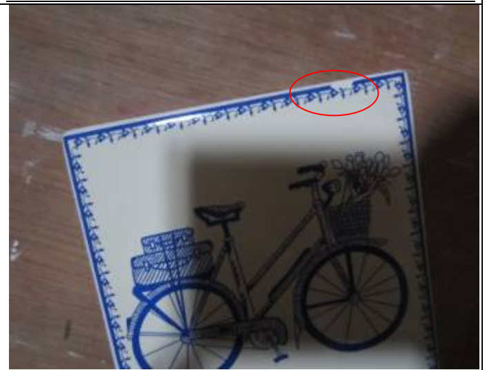
Decoration was not fully and poor painted
