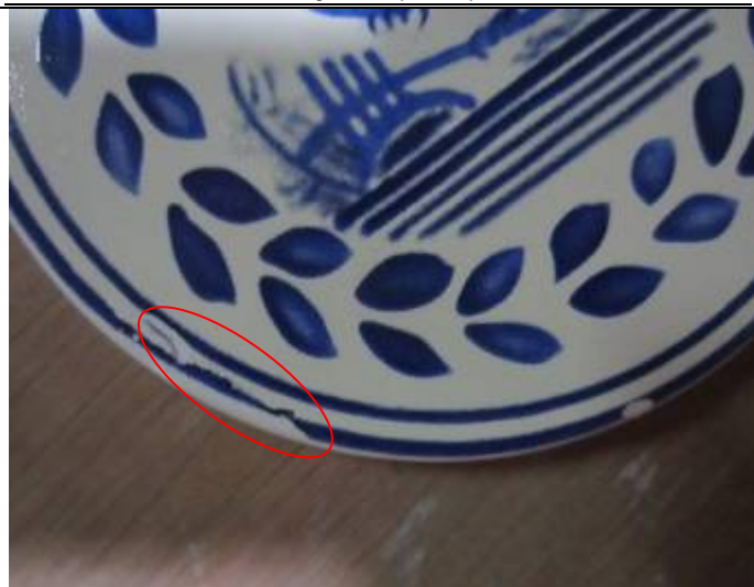
Decoration was not fully and poor painted
