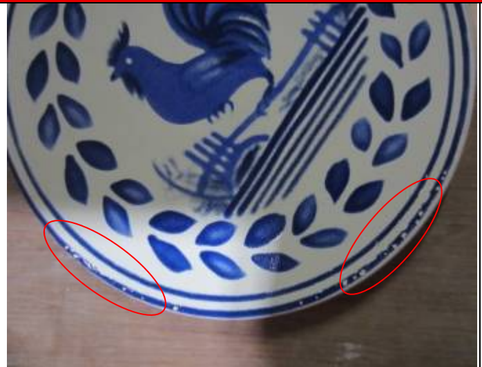
Decoration was not fully and poor painted
