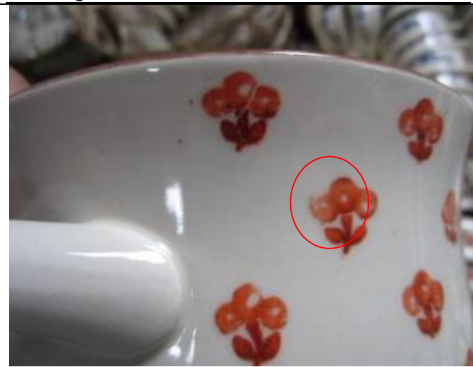
Decoration was not fully and poor painted
