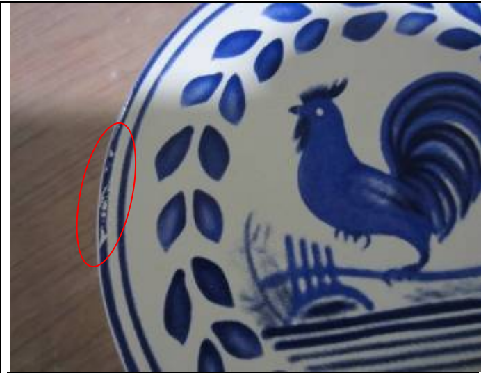
Decoration was not fully and poor painted
